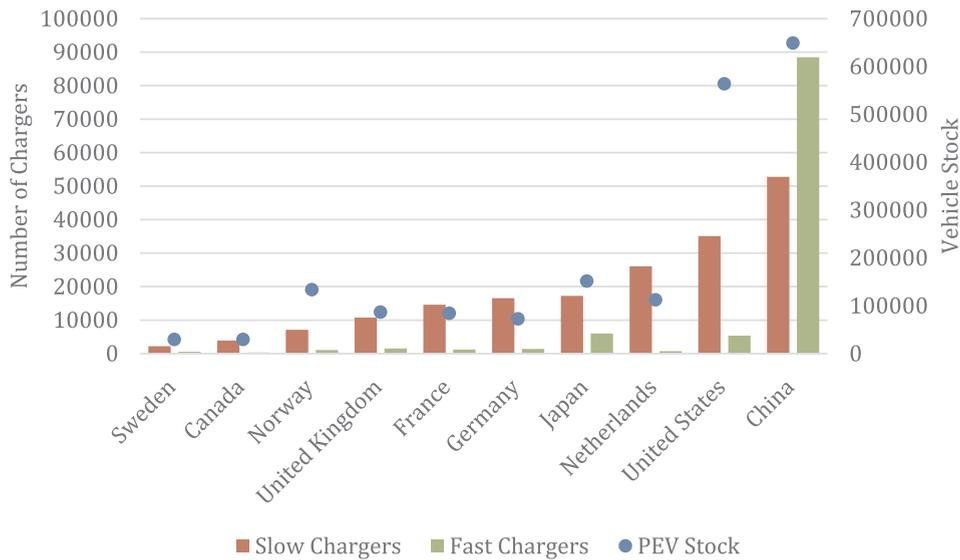
**Fig. 2.** Number of public slow (level 1–2) and DC fast chargers, and number of PEVs registered in the top 10 PEV markets. The number of charging stations differs between regions, and is related to the number of PEVs, travel patterns, housing type and other factors associated with local market conditions (International Energy Agency, 2017).
